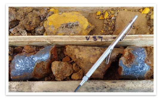
Figure 4. Galena mineralization with pervasive oxidation at 41m in hole MCH-22-002.
