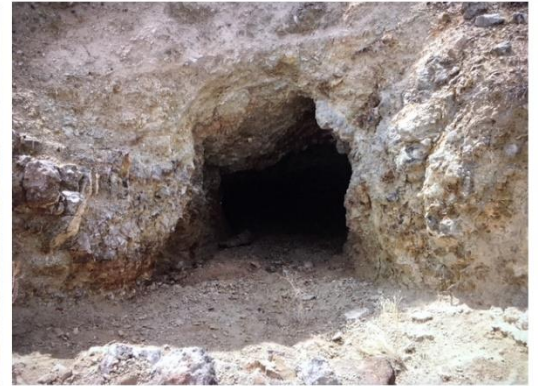
Adit into shallow dipping vein in limestone
