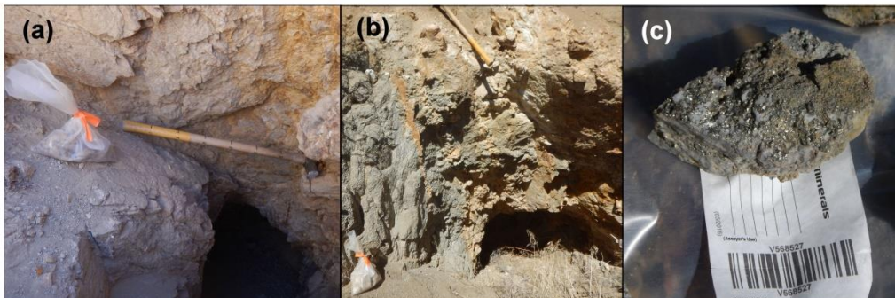
Loner mineralization (a) 0.3m @ 13.85 g/t Au from weathered vein (b) vein swarm in granite (c) sulphide mineralization at NW end of the property (10.2 g/t Au).
